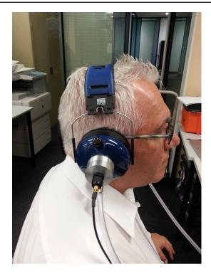
Fig. 14 Pneumatic driver constructed using earnuffs with attached tubing and low-frequency microphone [64]
