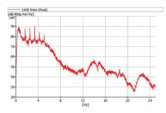
**Fig. 3** Measured infrasound power spectral density spectrum (1600 lines 0–25 Hz) showing a fundamental blade pass frequency of 0.85 Hz and harmonics recorded inside the bedroom of a residence located 1.6km from Cape Bridgewater Wind Farm, Victoria [32]
