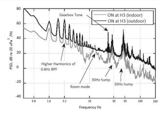
Fig. 11 Comparison between the indoor/outdoor power spectral density (dwelling H3) [33]
