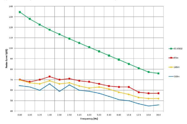
Fig. 7 Measured levels of infrasound at Clements Gap Wind farm with a hub height wind speed of 6-8 m/s [39]
